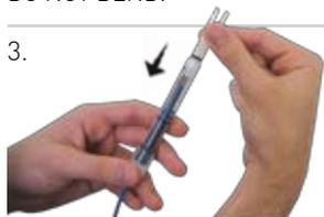
3. Slide the sleeve back onto the electrode ensuring the black O-ring is well seated within the electrode body. Do not exert sideways force. Any excess electrolyte will be expelled from the end of the electrode through the ground junction. Ensure there are no air bubbles in the sleeve. Wash off any excess electrolyte before use.
