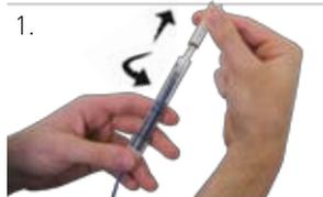
1. Invert the electrode. Hold the electrode just below the sleeve and with careful rotation and pulling along the axis of the electrode, remove the sleeve. DO NOT BEND.
