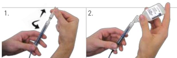
1. Invert the electrode. Hold the electrode just below the sleeve and with careful rotation and pulling along the axis of the electrode, remove the sleeve. DO NOT BEND.
